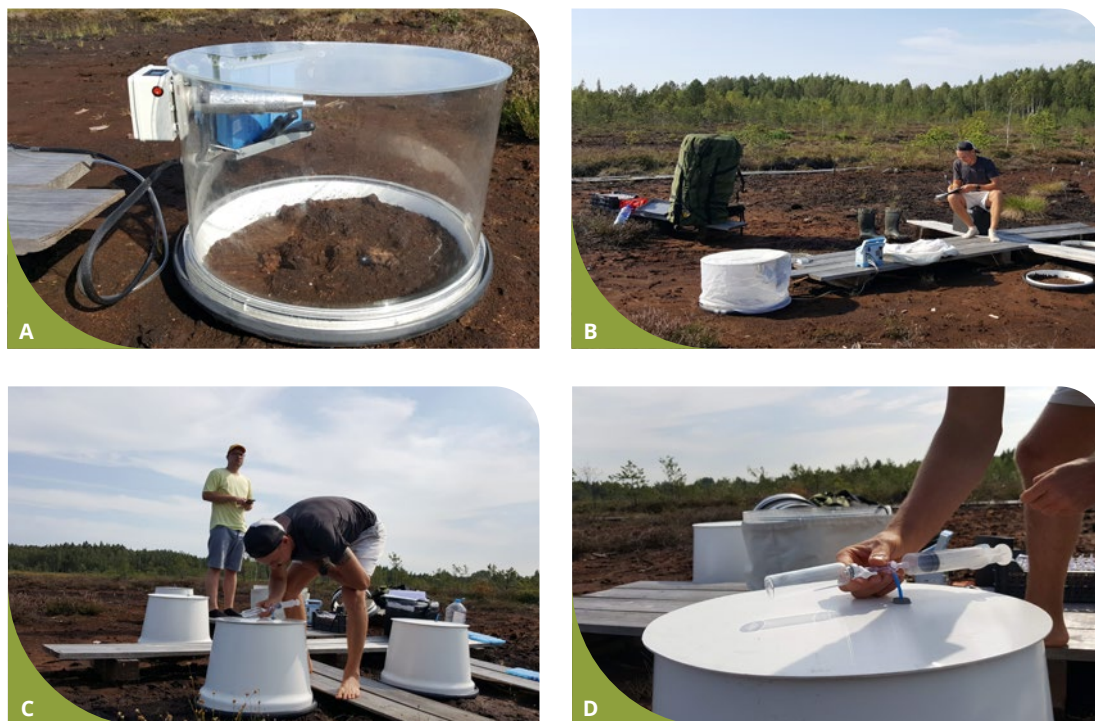
Figure 14. GHG measurements with transparent (A), shaded (B) and opaque (C–D) manual chambers in Püscia peatland. Photos: J. Sendžikaite.
